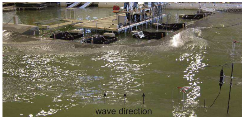
Figure 2. Dike model with overtopping units behind the dike during a test.
