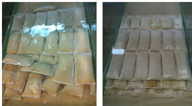
Figure 2. Stability tests: (a) original and (b) modified configuration ( H_i=0.075 m, T=1.6 s at laboratory scale).
