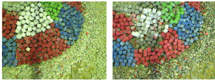
Figure 2 Damage in the armour layer for the 2 nd typology tested (Initial –Left– and resulting –Right– state of the roundhead).
