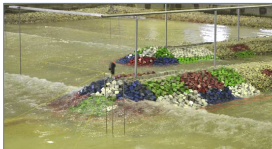
Figure 1 The two adjacent breakwaters at the CITEEC wave tank
